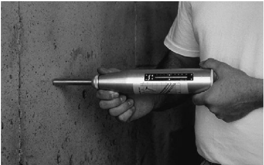
Figure 9.6 Rebound number determination using a “rebound hammer.” Courtesy of Portland Cement Association.
