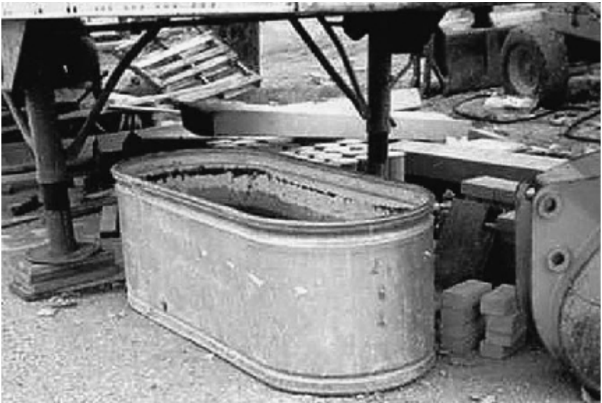
Figure 9.12 Initial jobsite curing by immersion in lime-saturated water. Cylinders in background represent previous, problematic initial curing conditions.
