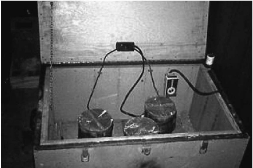
Figure 9.3 Temperature controlled jobsite-curing box. Courtesy of CTLGroup.
